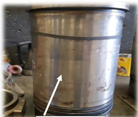
Cracked cylinder liner
