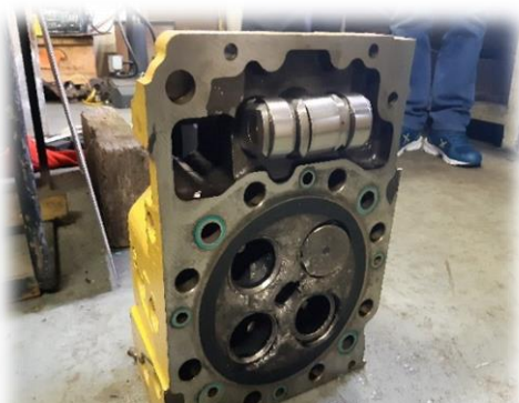
Damage on one cylinder head unit
